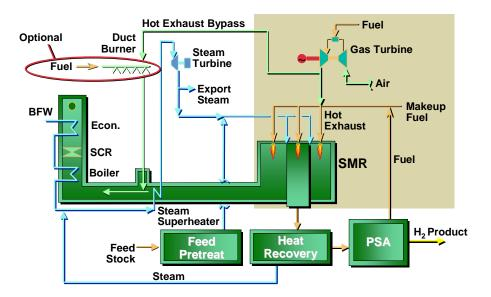
The steam system in the hydrogen plant is upgraded above 45 barg to 105 barg. All the high-pressure steam generated is sent to the topping turbine for power recovery before process use for the reforming reaction and export to the refiner. Appropriate bypasses can be incorporated into the plant design to de-couple hydrogen and steam production from power production.
